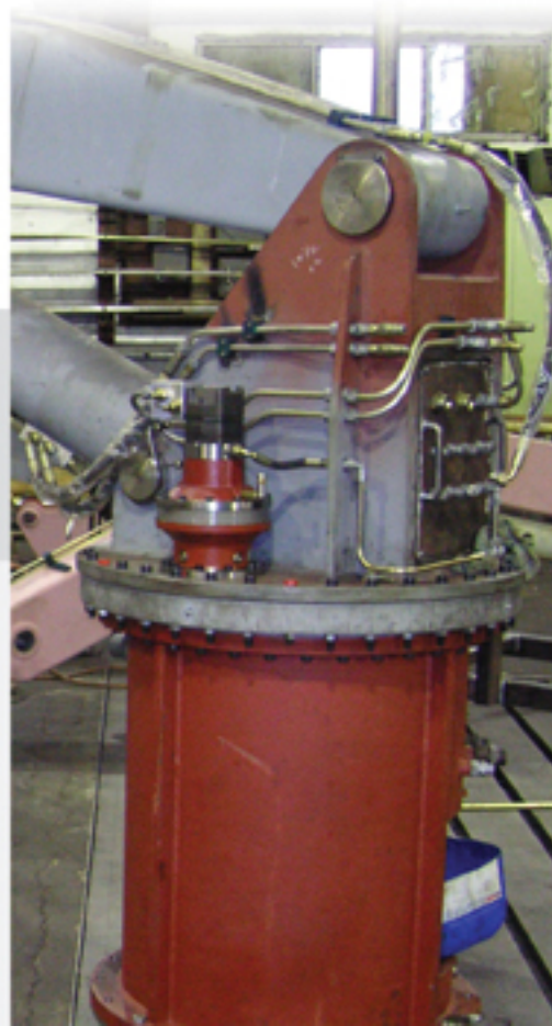
↘ Pedestal Crane base under construction at our machine shop.
