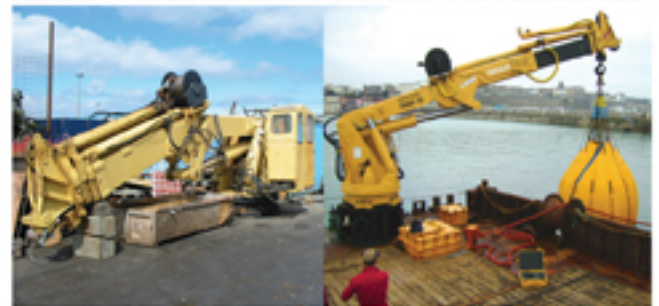
↗ Effer 110T/mt workbarge crane before and after full refurbishment.
