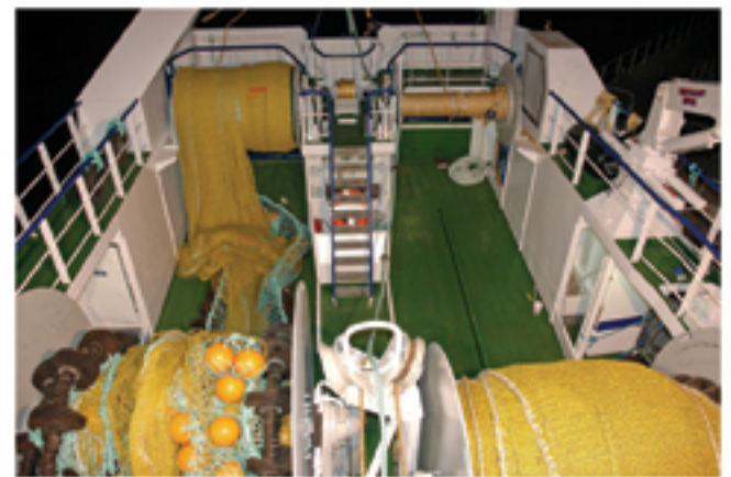
↗ Aft Deck - view of split Net Drums on Lunar vessel rated 15 Tonne Core Pull.
